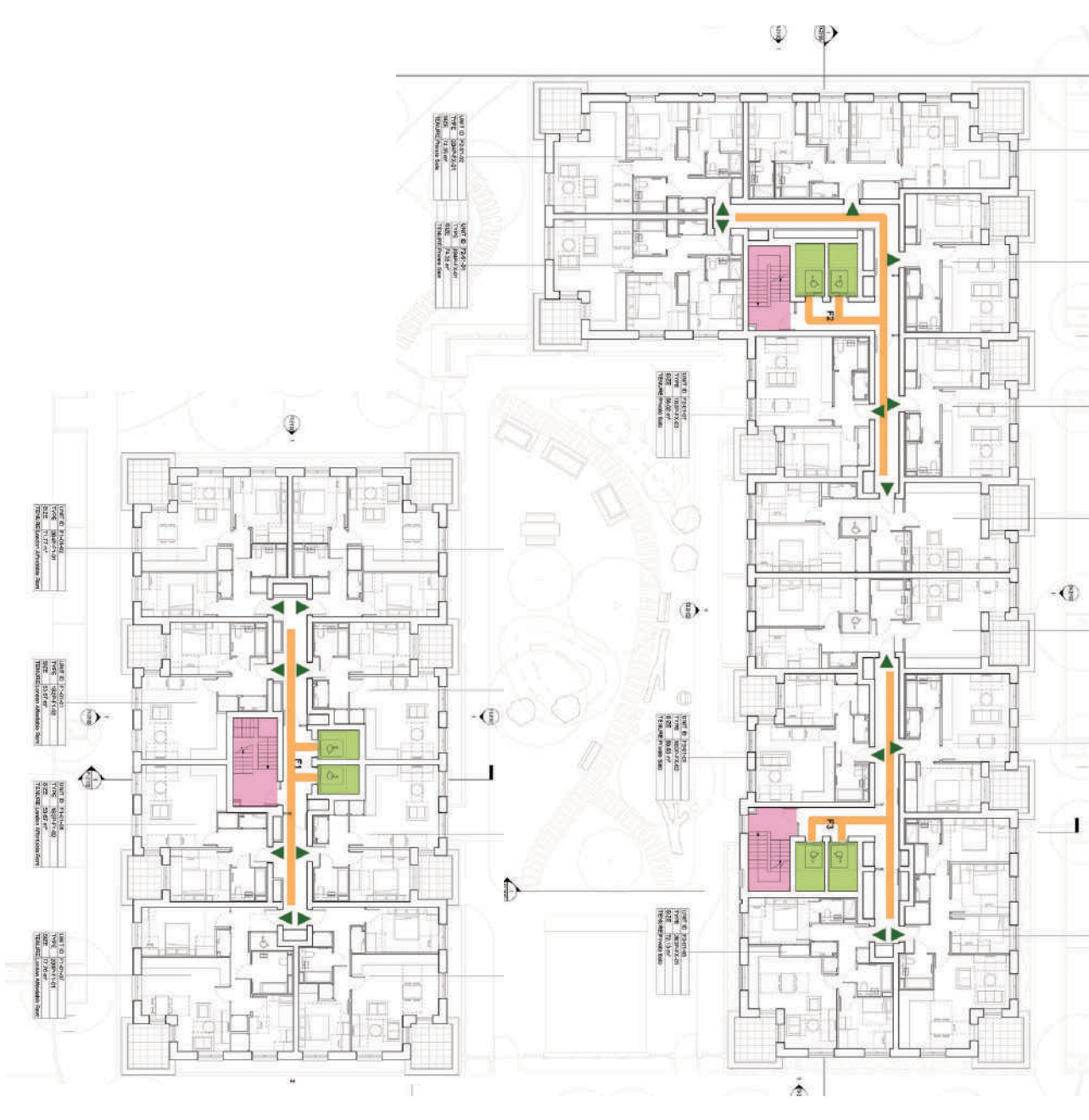
Fig.6 Building F - Proposed Typical floor - Access overlay
