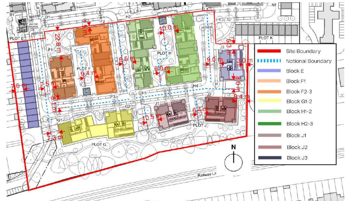
Figure 23: External Fire Spread Assessment
