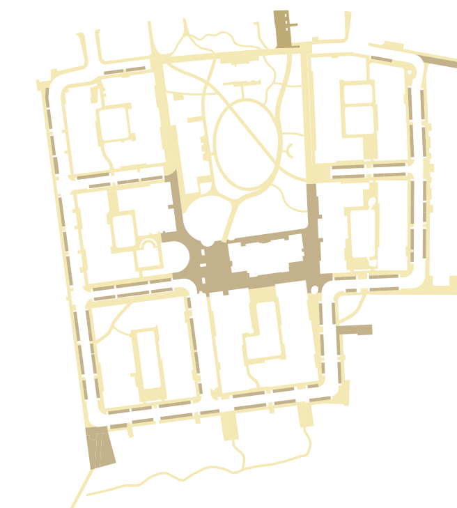
Extent of permeable paving
