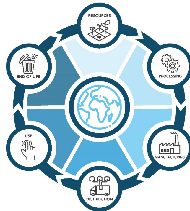
Figure 1: Stages included within an LCA.
