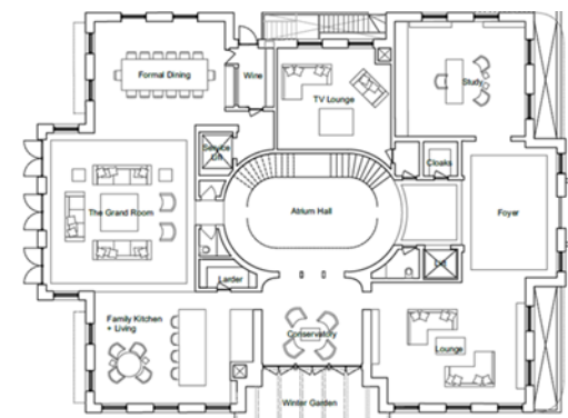
Figure 1b: Proposed ground floor plan of the scheme
