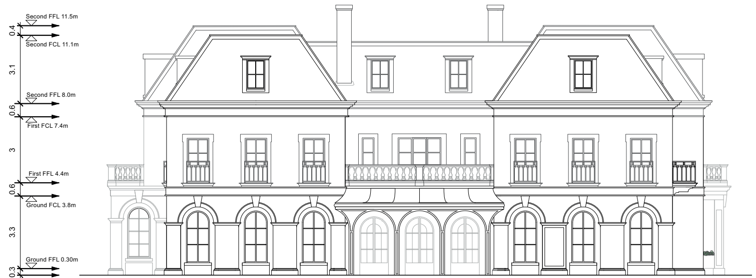
Figure 36. Previously proposed building levels
