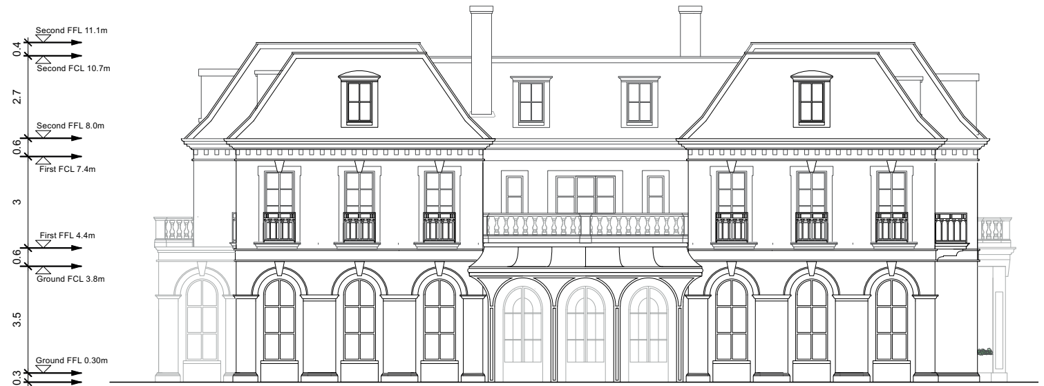
Figure 35. Final building levels
