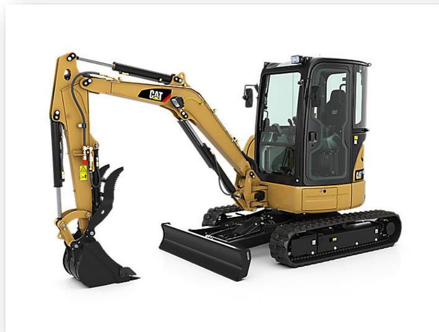
Small Excavator used near Boundaries
