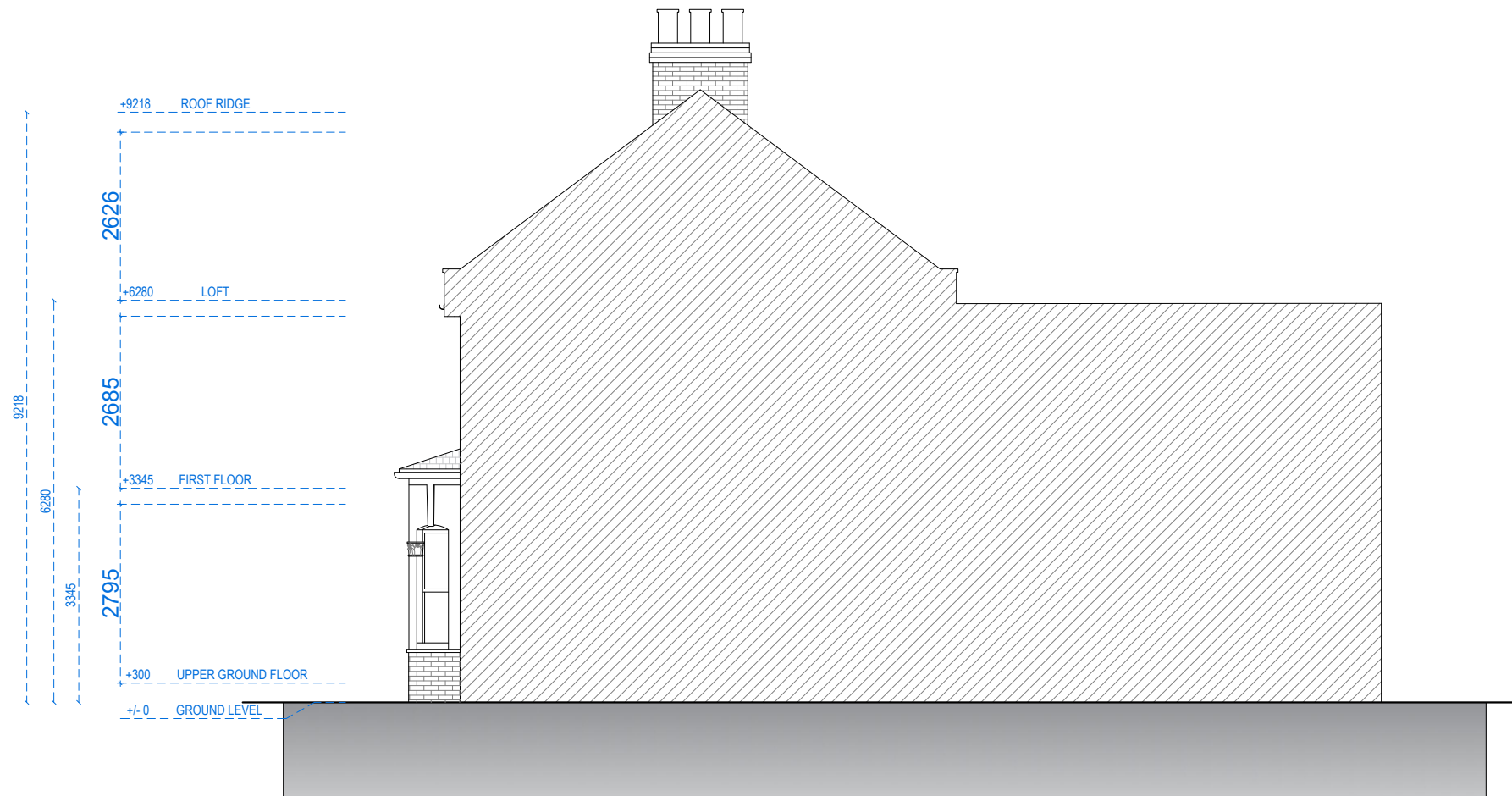
SIDE ELEVATION EAST ELEVATION
