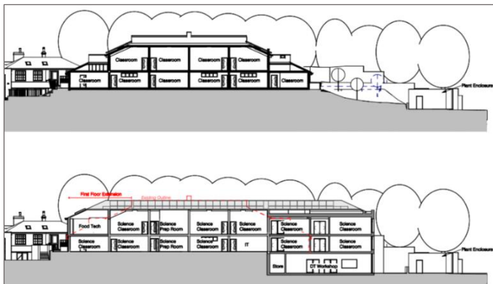
Figure 3: Brunner House Existing and Proposed Sections
