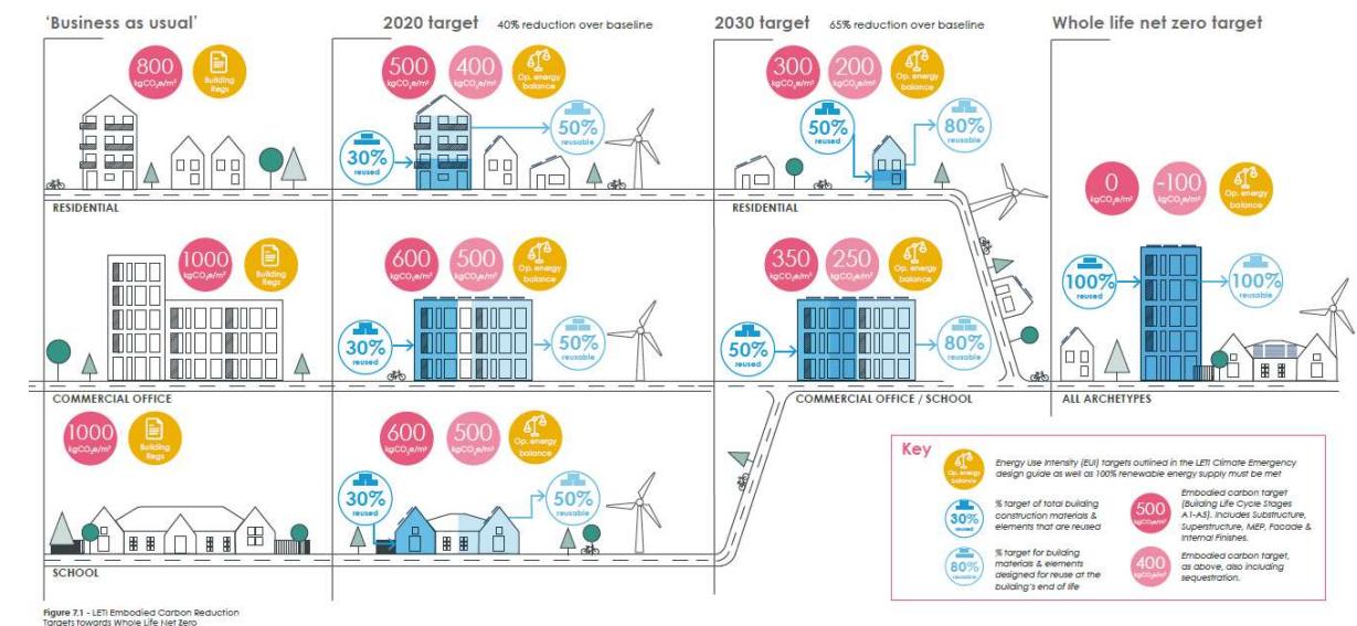
Figure 17: Targets for Achieving Net-Zero Carbon from "Embodied Carbon Primer" (LETI, 2019)
