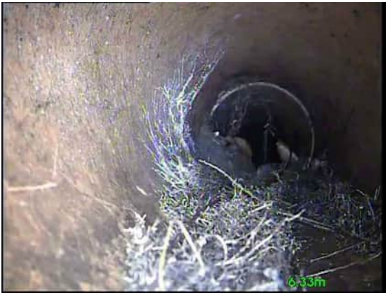
9, 00:00:55, 6.33 m Roots, mass, 35% cross-sectional area loss, change
