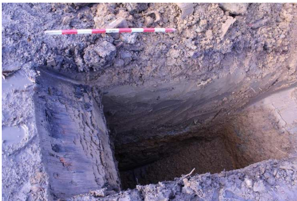
Plate 2: Machine excavated Test Pit 2: Made ground, Enfield Silts brickearth Kempton Park Gravels and top of London Clay.
