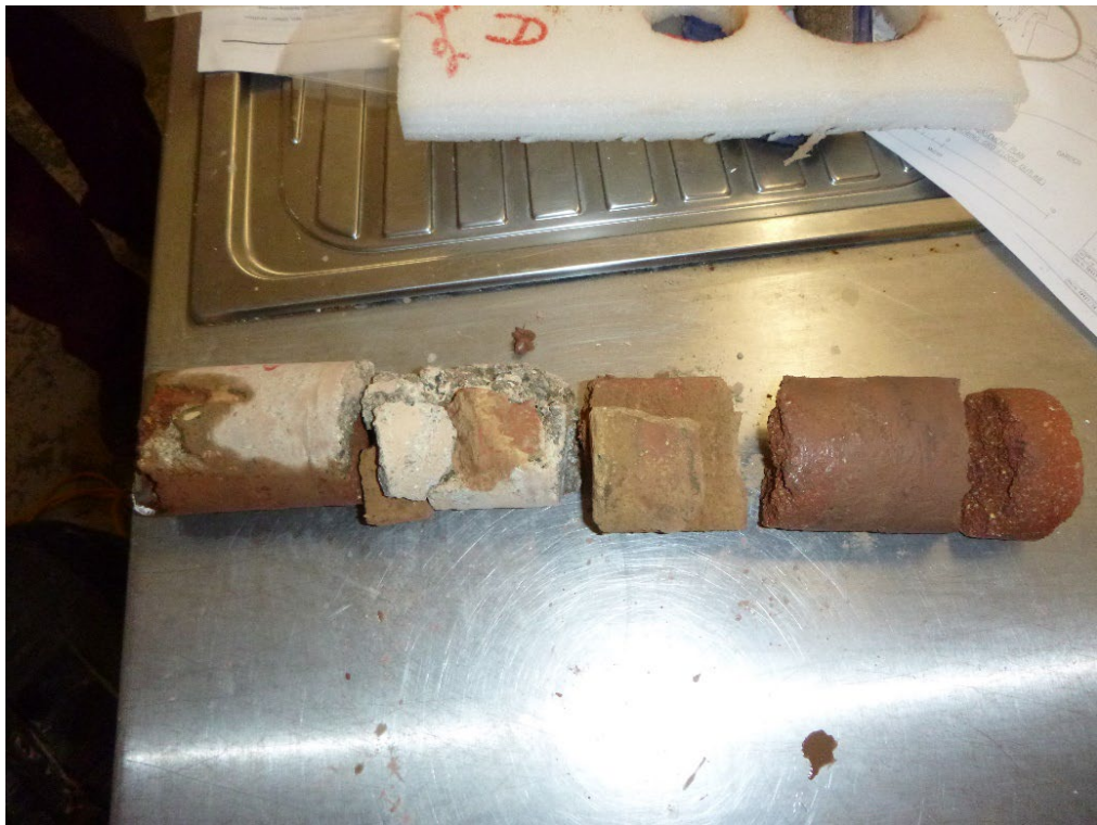
Photograph 6 Location A2. Core sample. Well filled.
