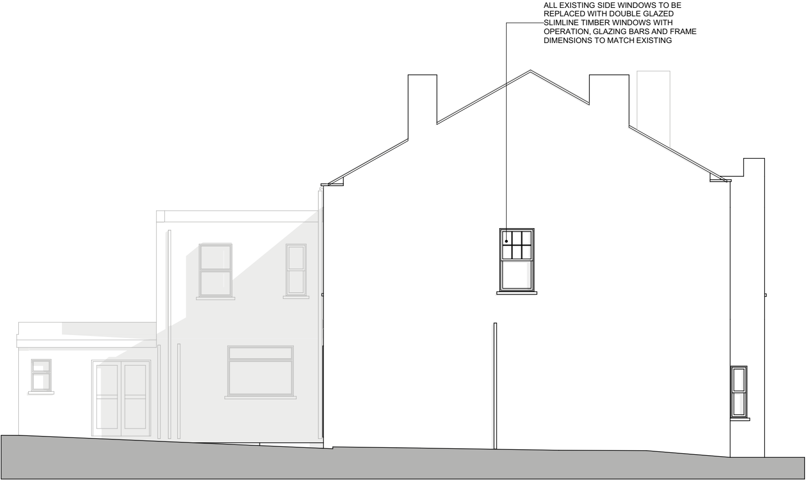
1 Existing Side Elevation 1:100
