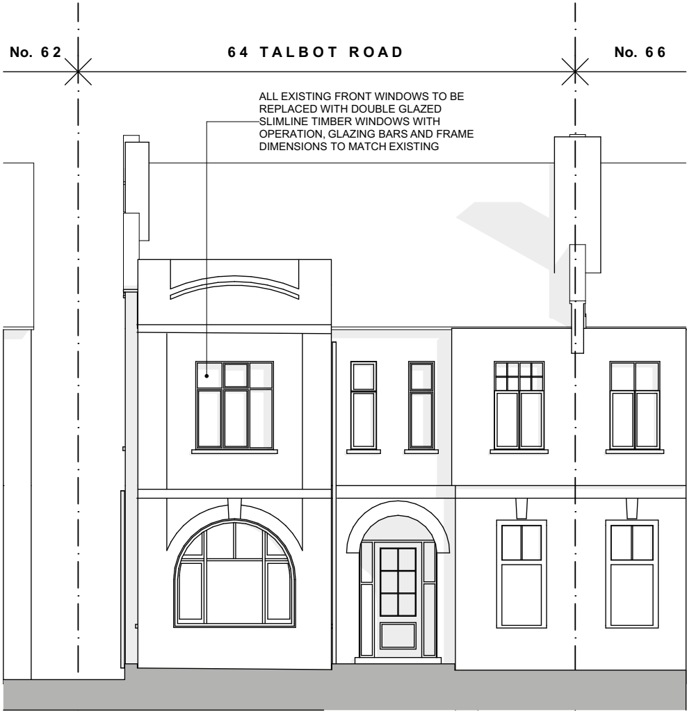
1 Existing Front Elevation 1:100
