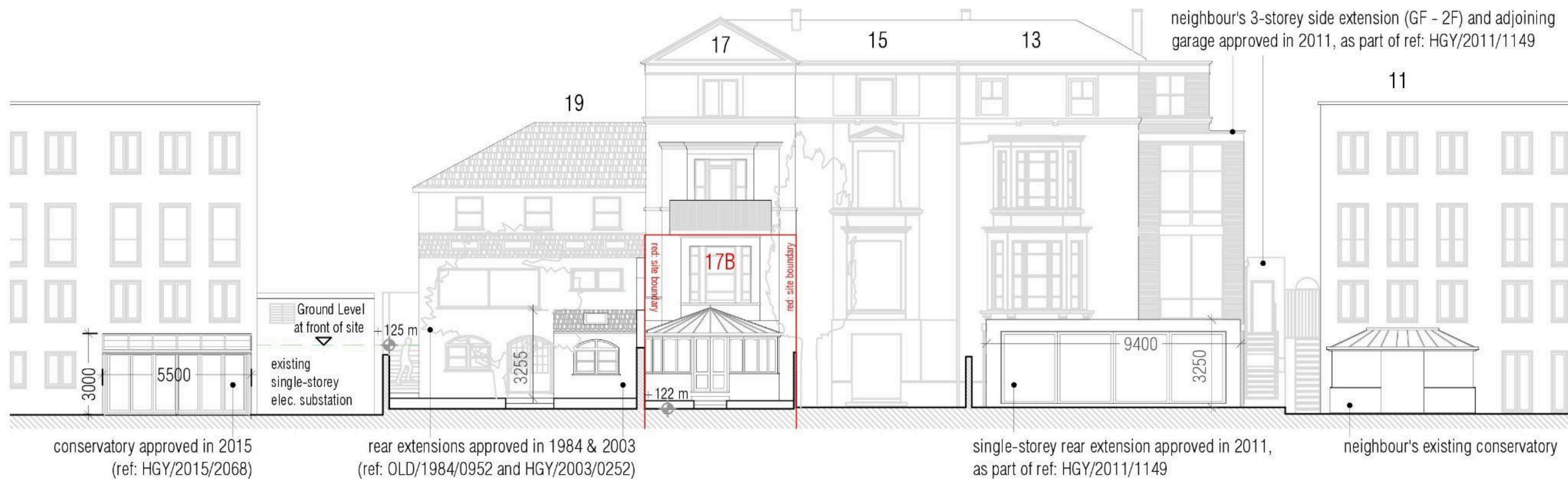
Existing Rear Block View showing heights and extent of extensions/conservatories along terrace and neighbouring blocks (details in drawing 0-012 submitted)
