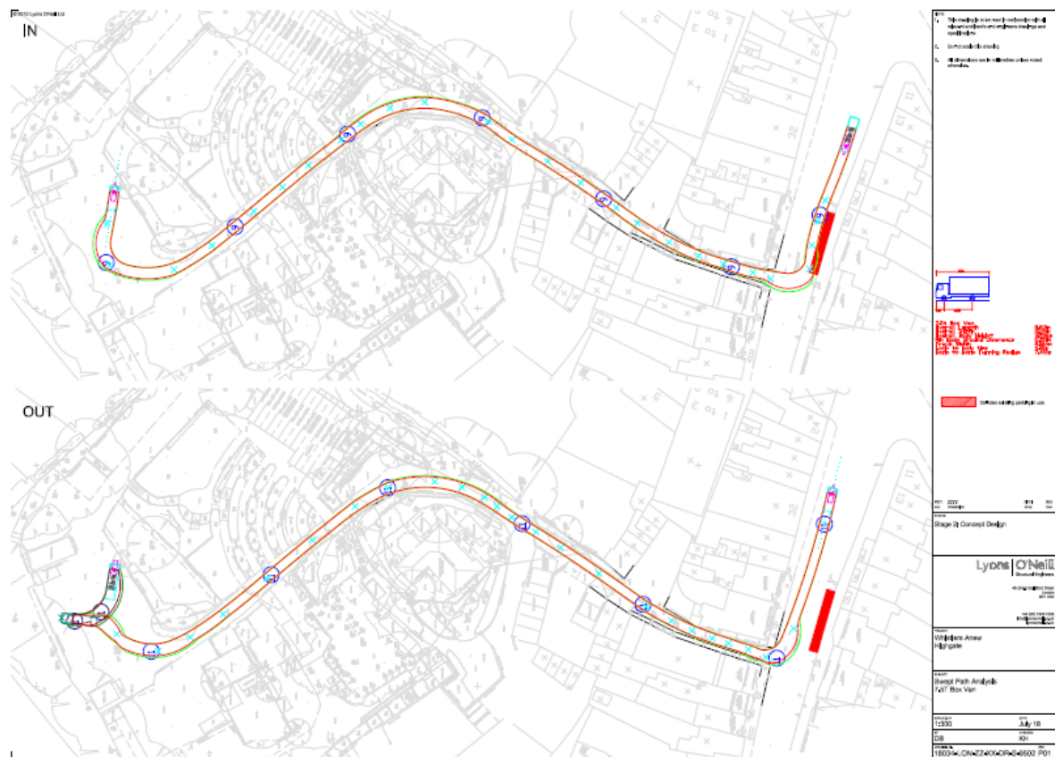
Proposed Traffic/Delivery Arrangements * (note: Vehicle turning will take place close to the entrance gates to OmVed Gardens as Appendix A)
