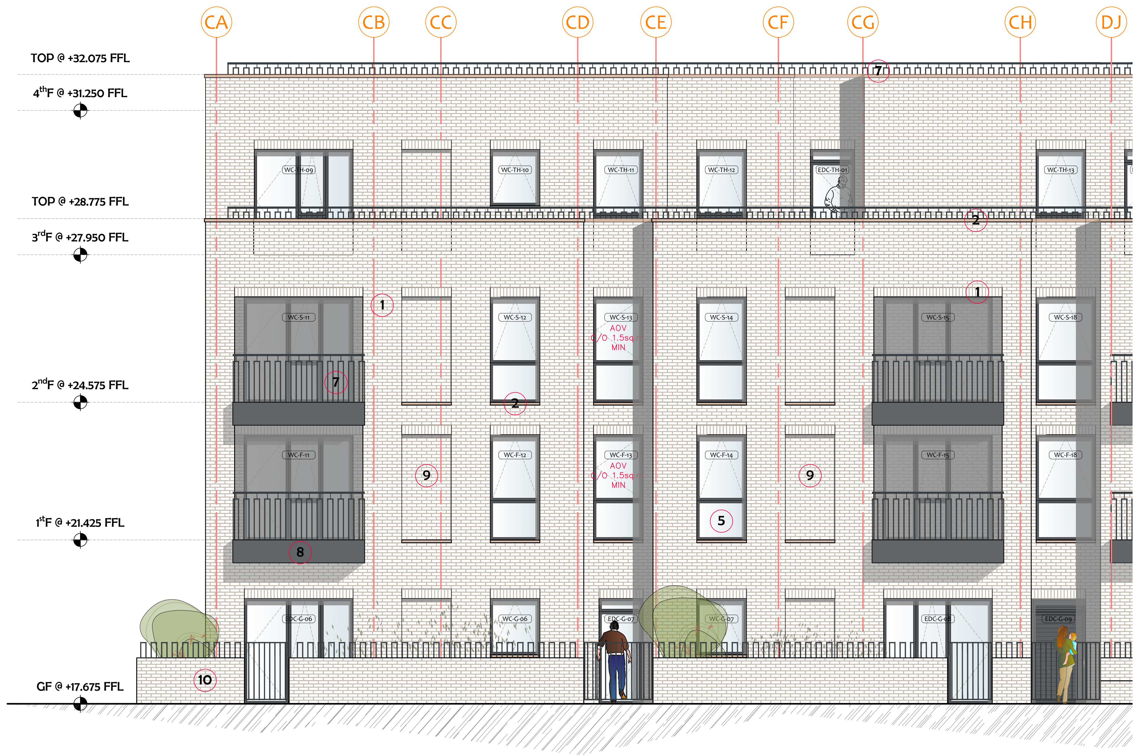
Proposed East Elevation (Church Ln) - BLOCK C 1:50@A1
