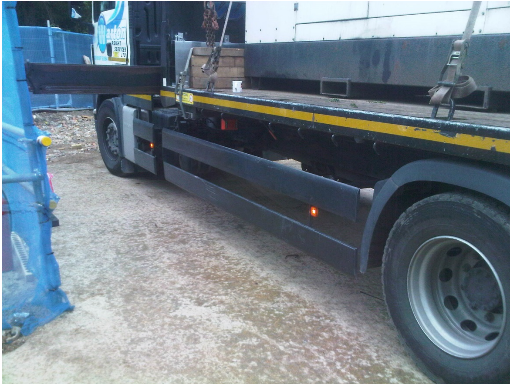
Above shows mirrors required, below full side rails
