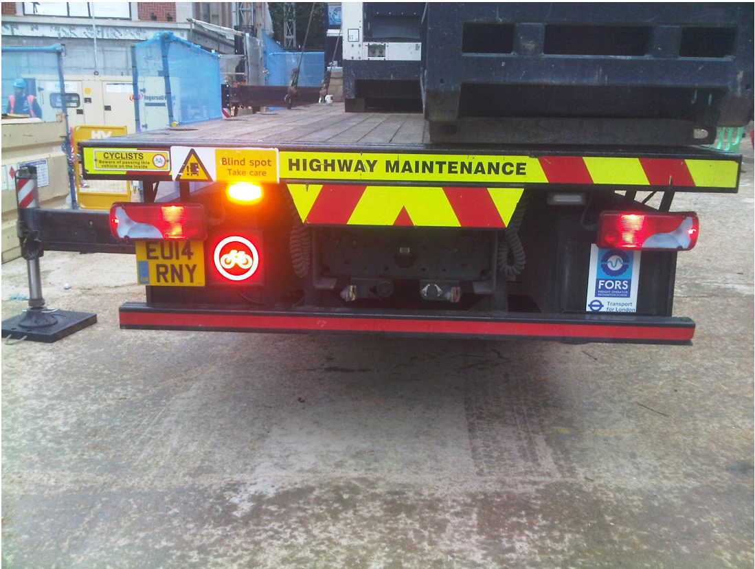
Above is the illuminated cyclist warning sign on the LHS. Note the FORS silver class signage on the RHS. Below the different mirror classes are explained
