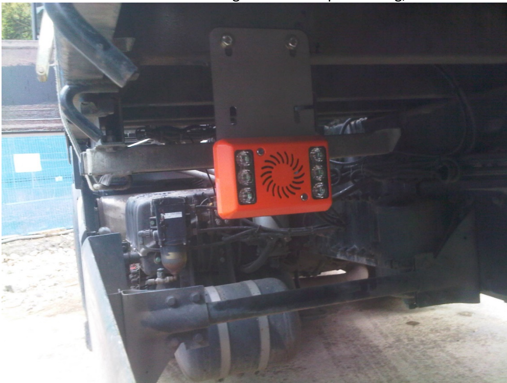
Above shows side indicator warning when blind spot turning, below a close up of the sounder
