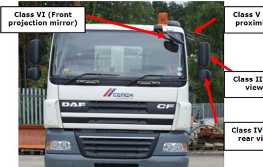
Below are images of FORS gold class vehicles, NS cyclist and pedestrian protection is enhanced.
