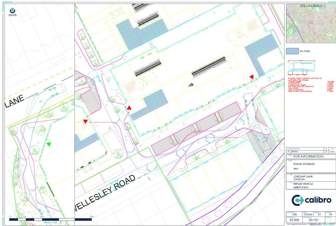
Figure 2-4 Refuse Vehicle Swept-path Analysis
