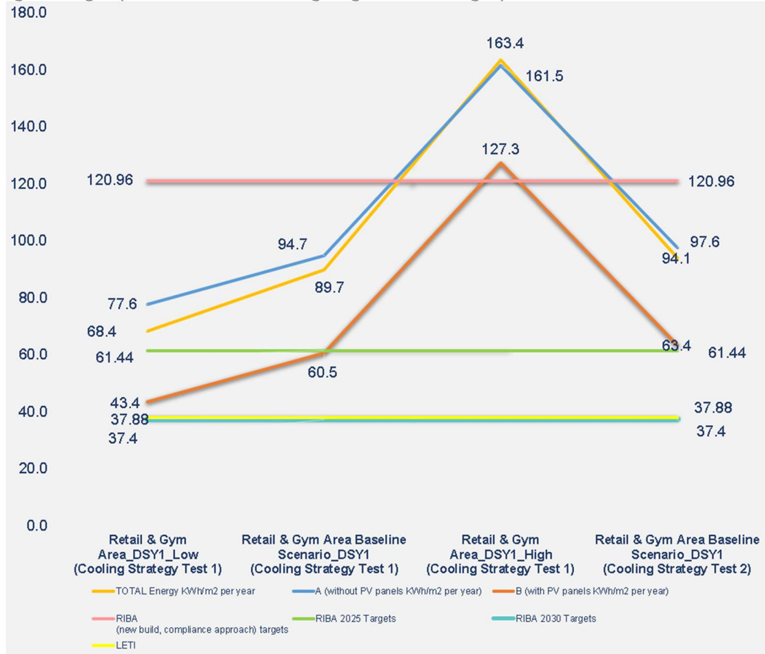
Figure 10.14. Lordship Lane Energy Consumption – Comparing “Low”, “Medium”, “High” DSY1 scenarios against Targets (RIBA 2030 Climate Challenge targets and LETI targets)
