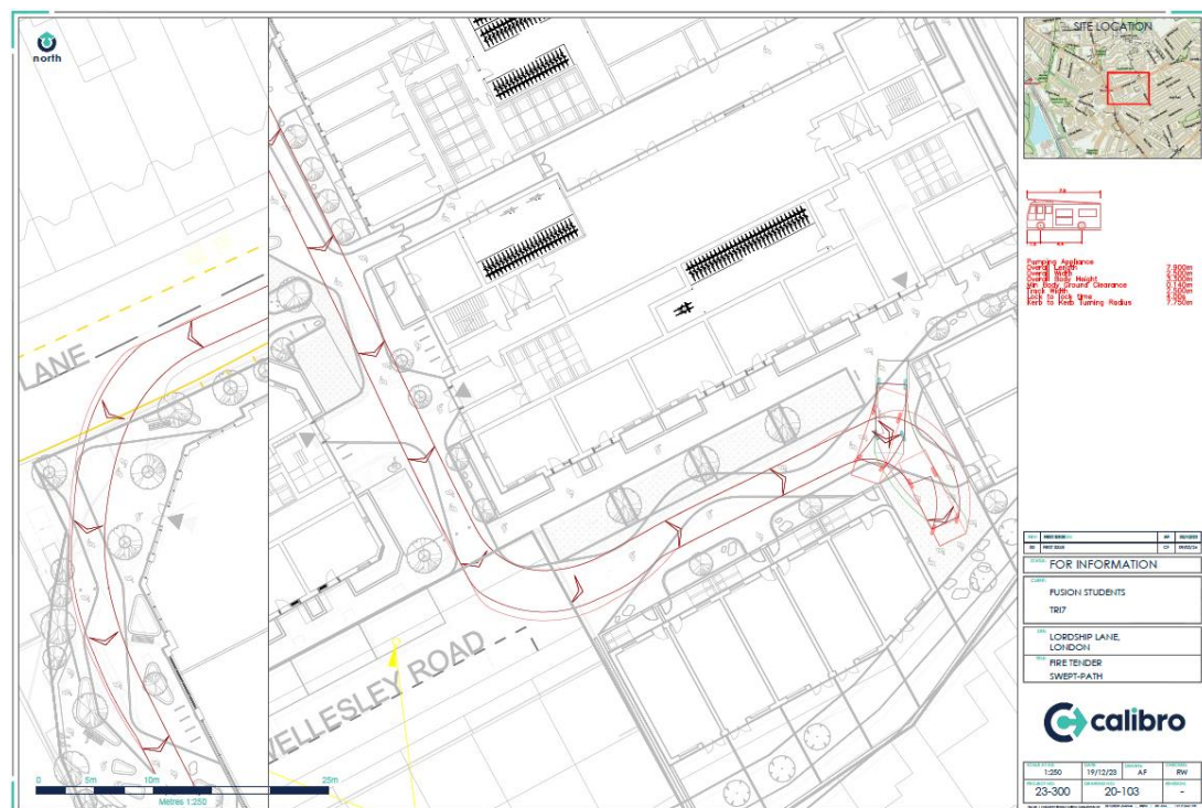
Figure 3-4 Fire Tender Swept Path Analysis
