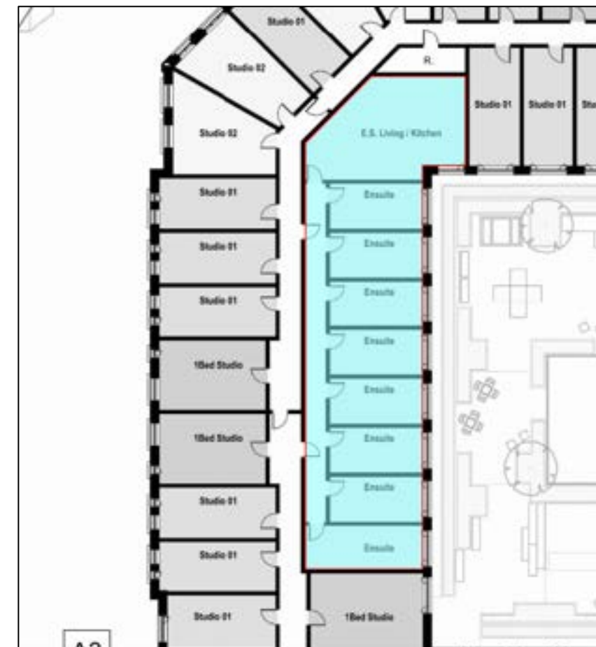
Figure 55: Cluster Accommodation Example
