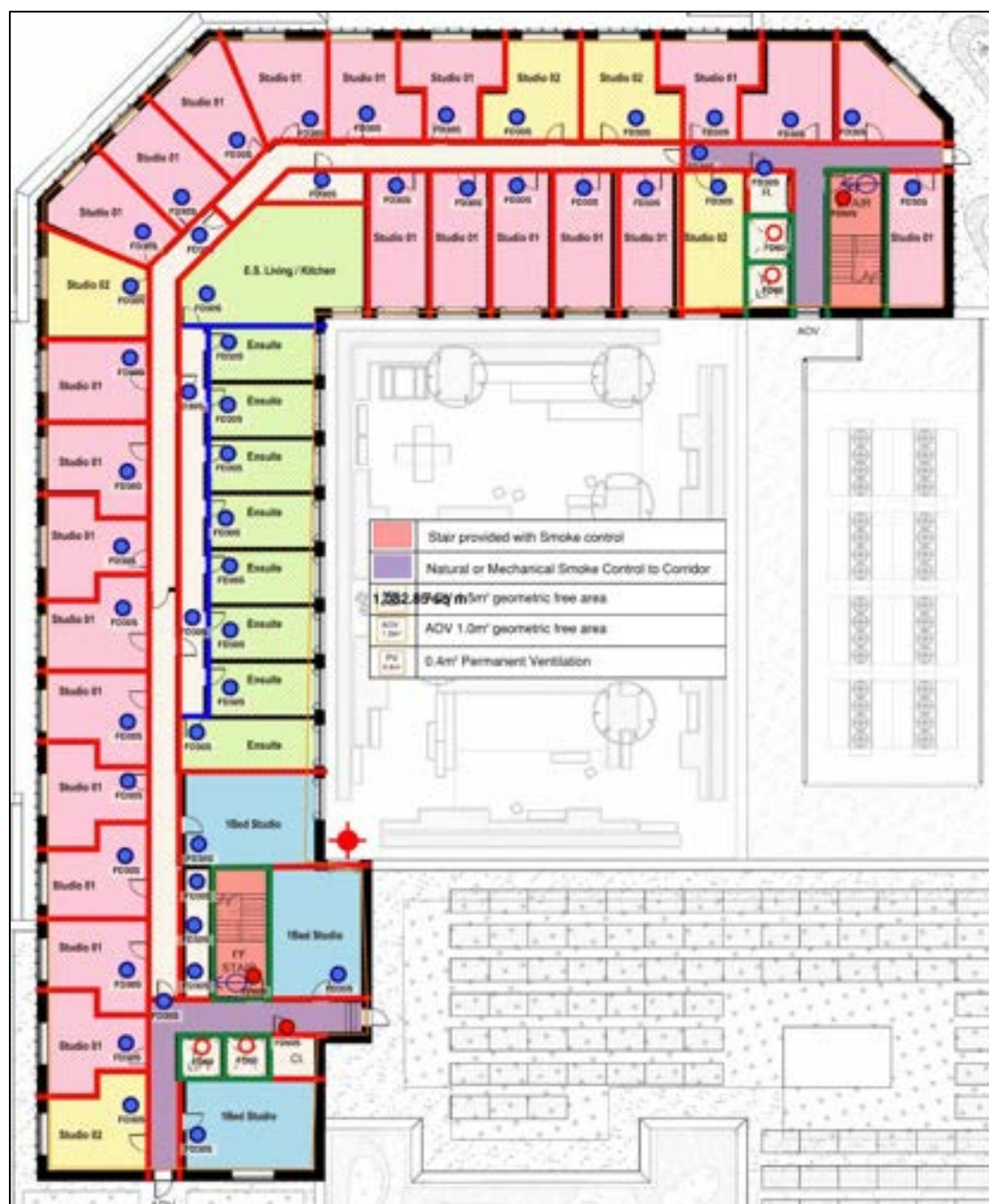
Figure 48: Floor 8 Smoke Control Summary
