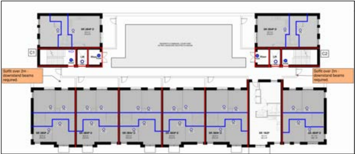
Figure 43: Balcony Escape Building C
