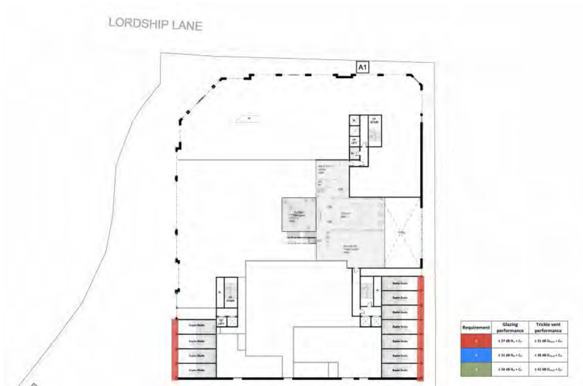
Figure 12: Façade acoustic performance requirements – Block A Mezzanine
