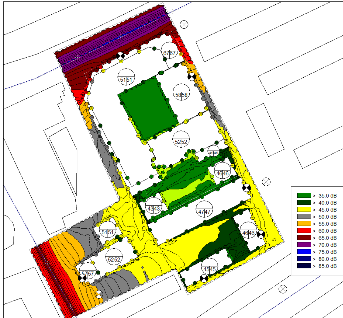
Figure 4: Night-time L_{Aeq, 8\text{ hr}} sound contours at 1.5 m above ground
