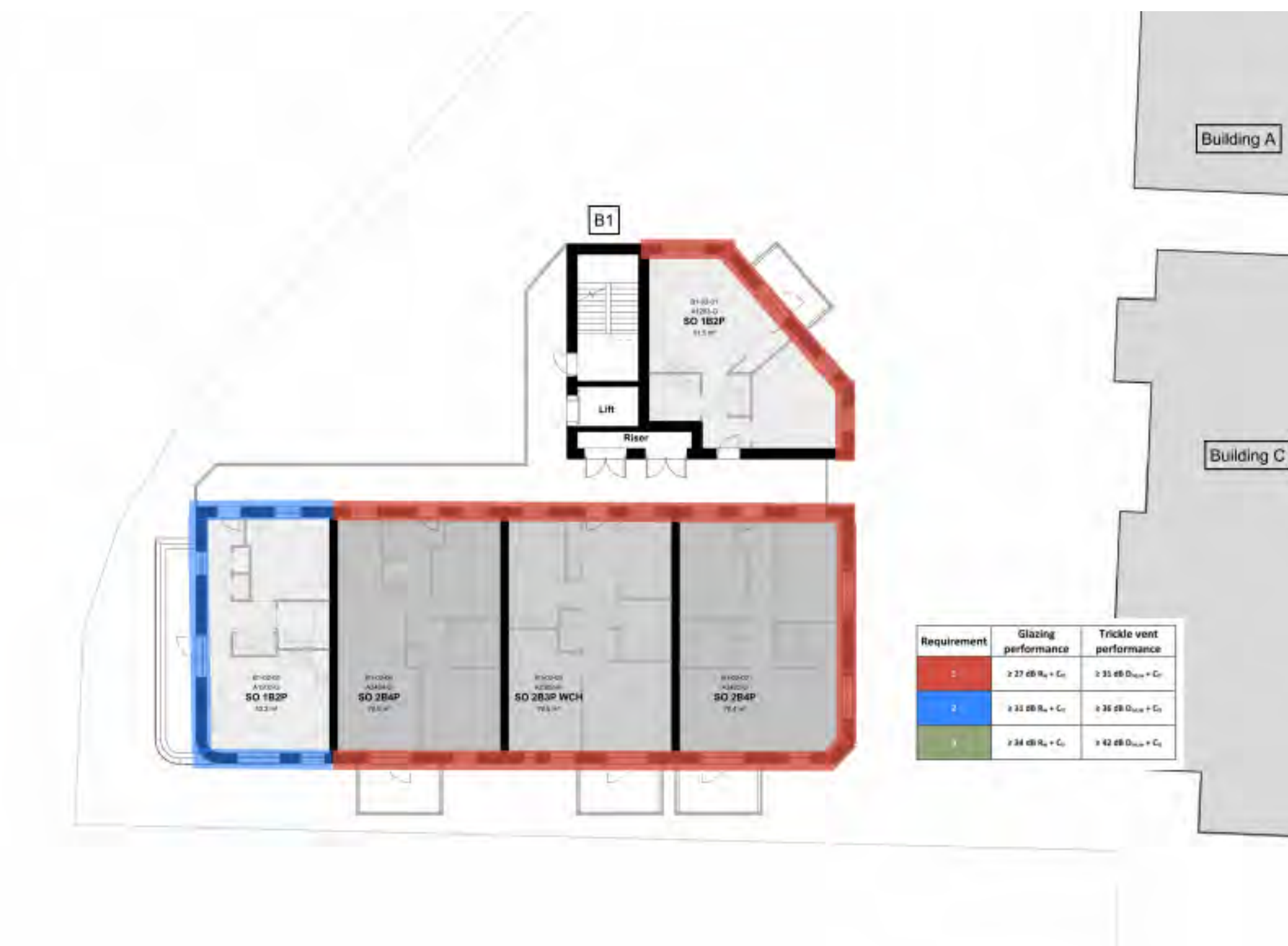
Figure 19: Façade acoustic performance requirements – Block B Level 02 to 04
