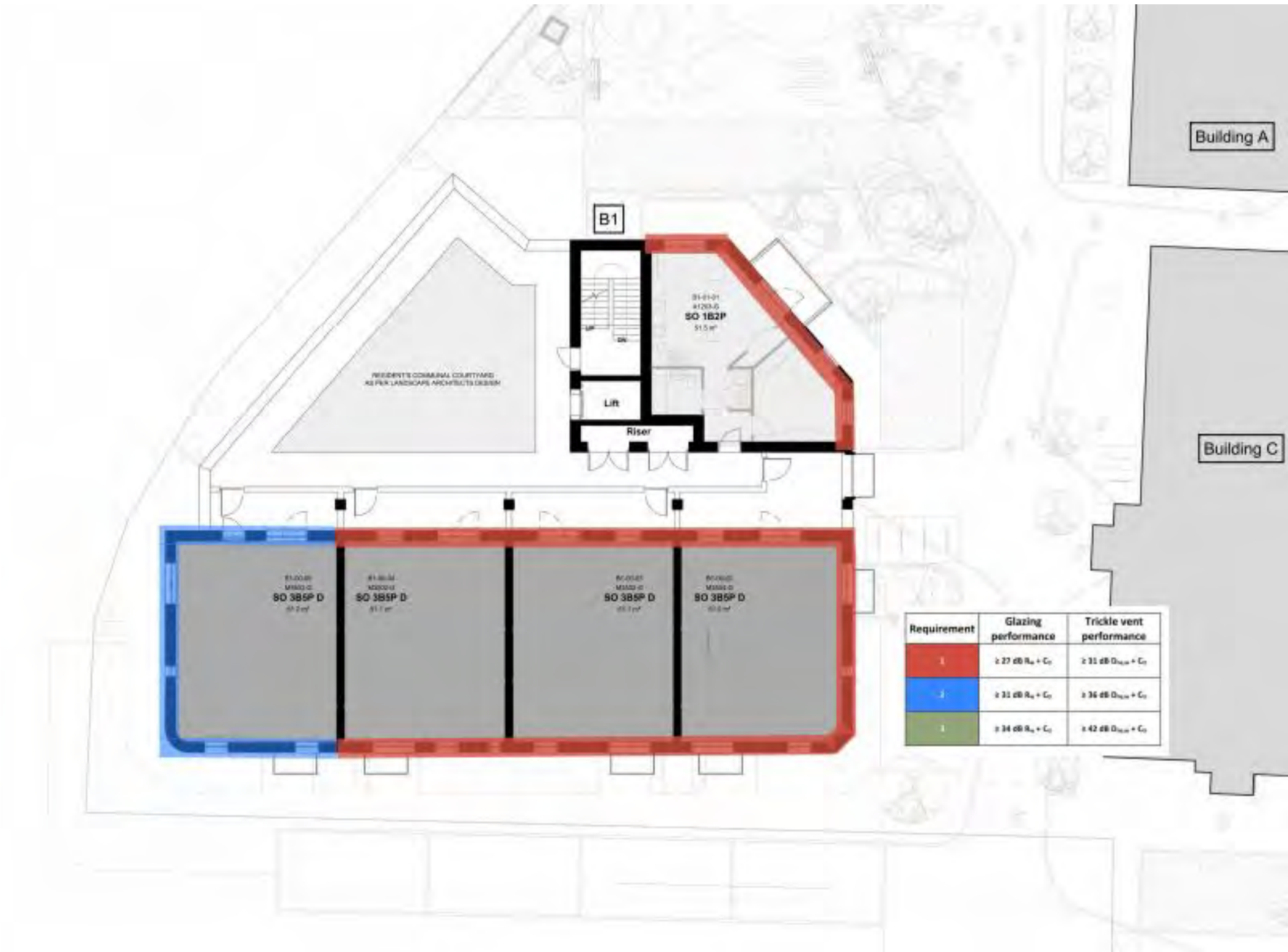
Figure 18: Façade acoustic performance requirements – Block B Level 01
