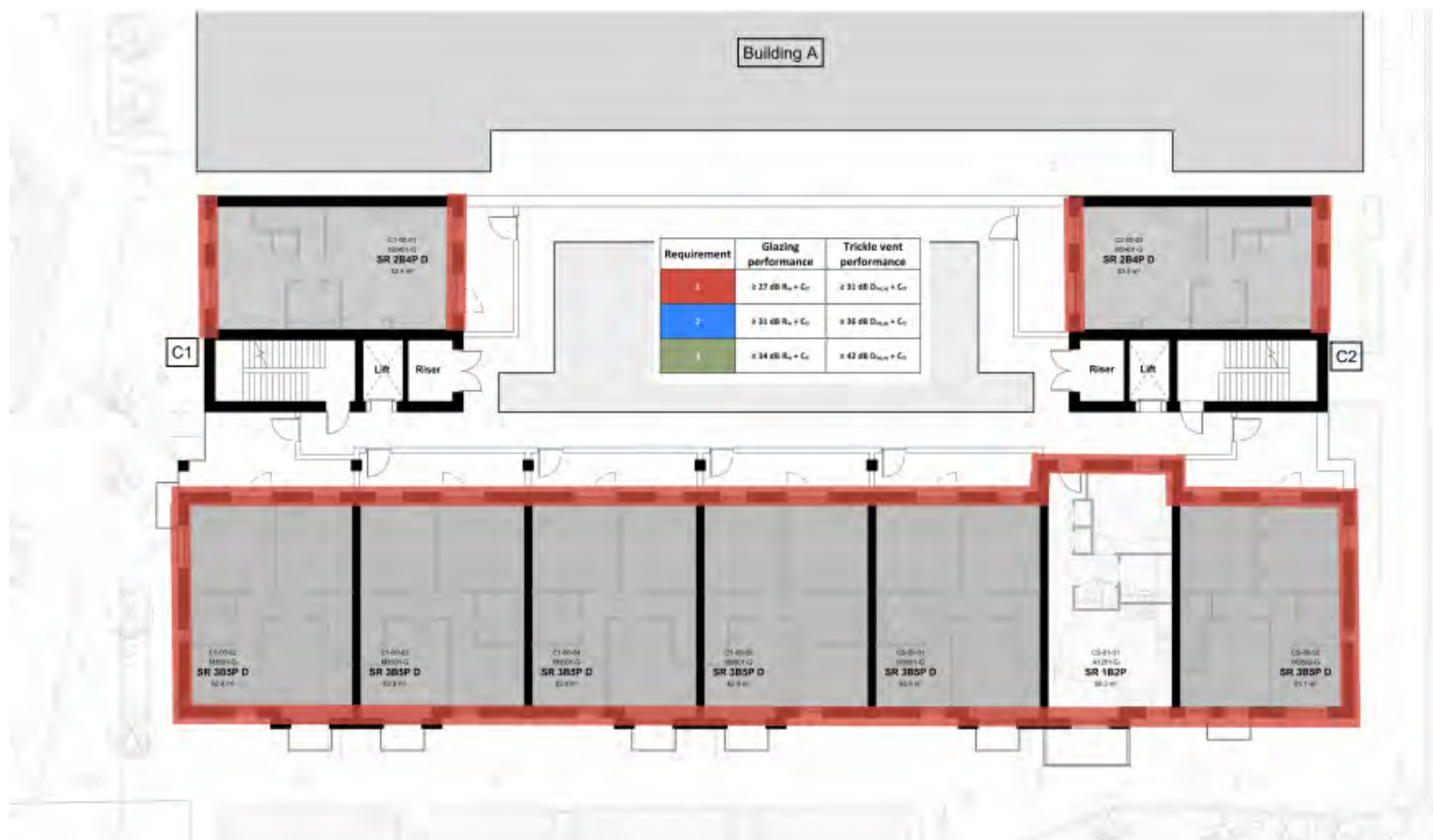
Figure 22: Façade acoustic performance requirements – Block C Level 01
