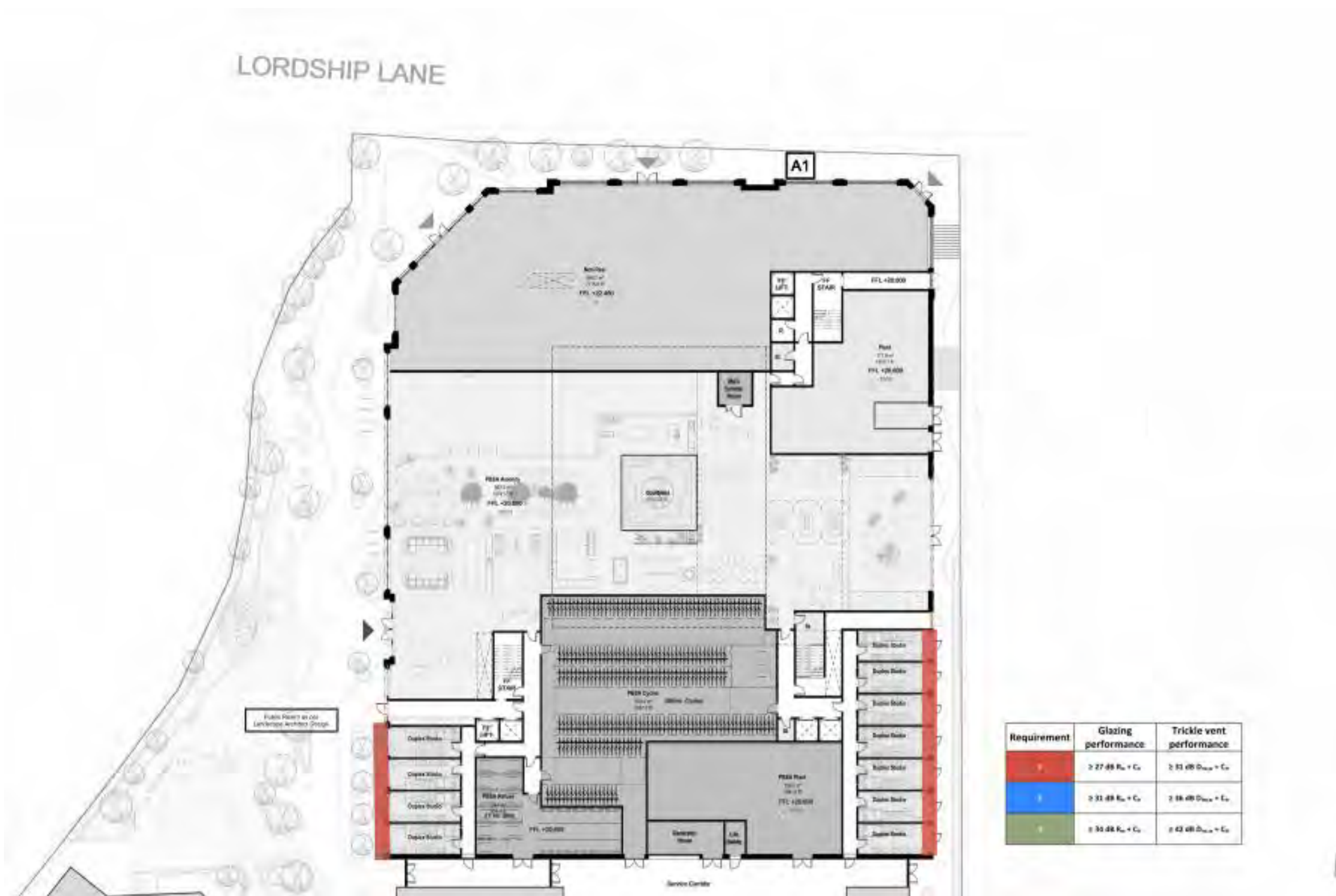
Figure 11: Façade acoustic performance requirements – Block A Level 0
