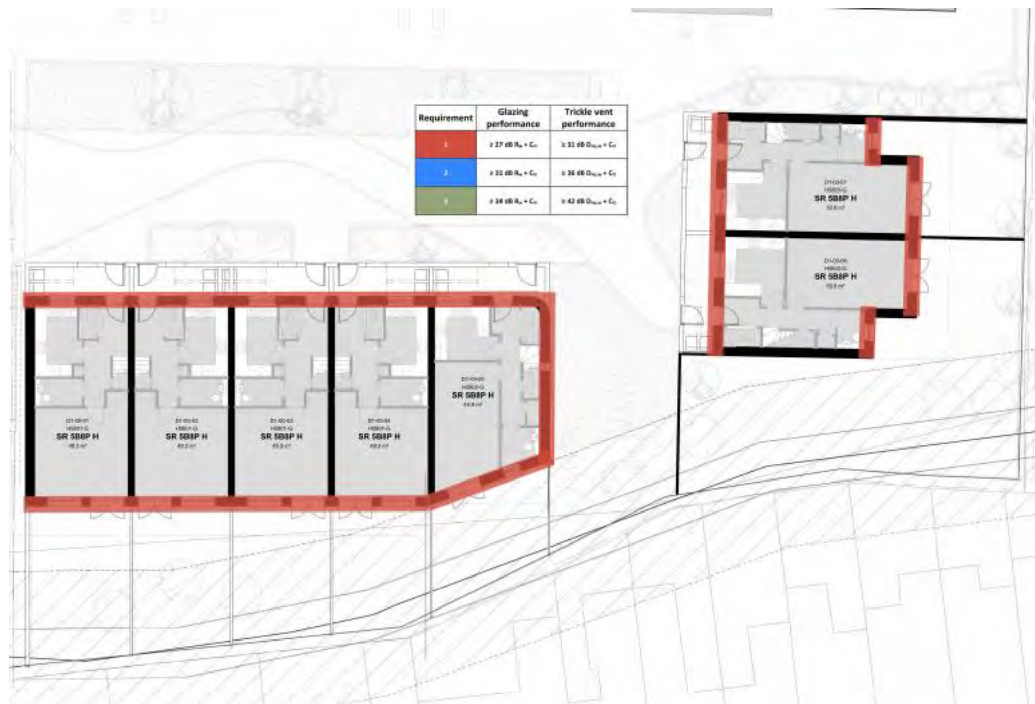
Figure 24: Façade acoustic performance requirements – Block D Level 00
