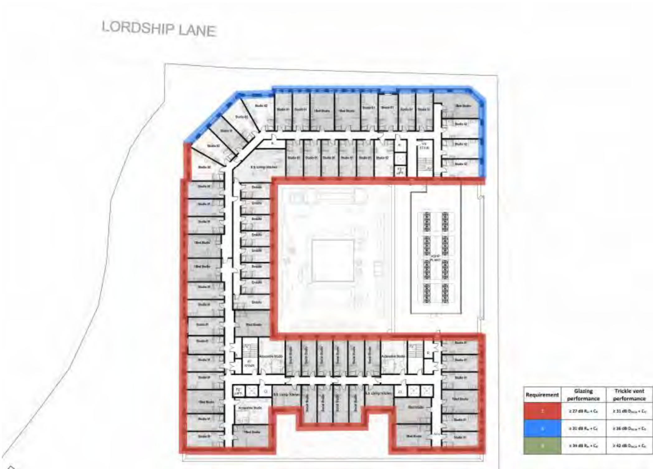
Figure 15: Façade acoustic performance requirements – Block A Level 07
