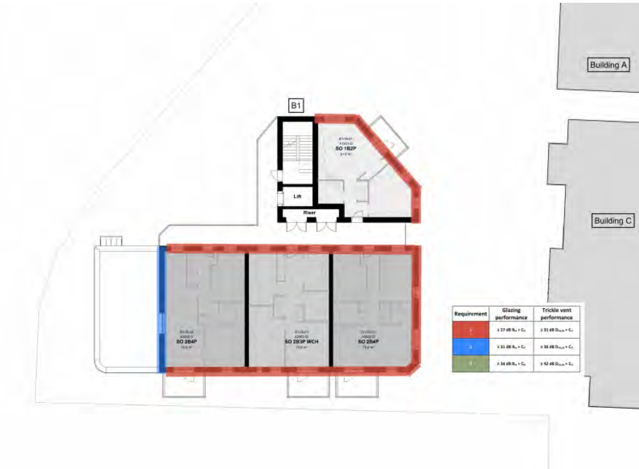
Figure 20: Façade acoustic performance requirements – Block B Level 05
