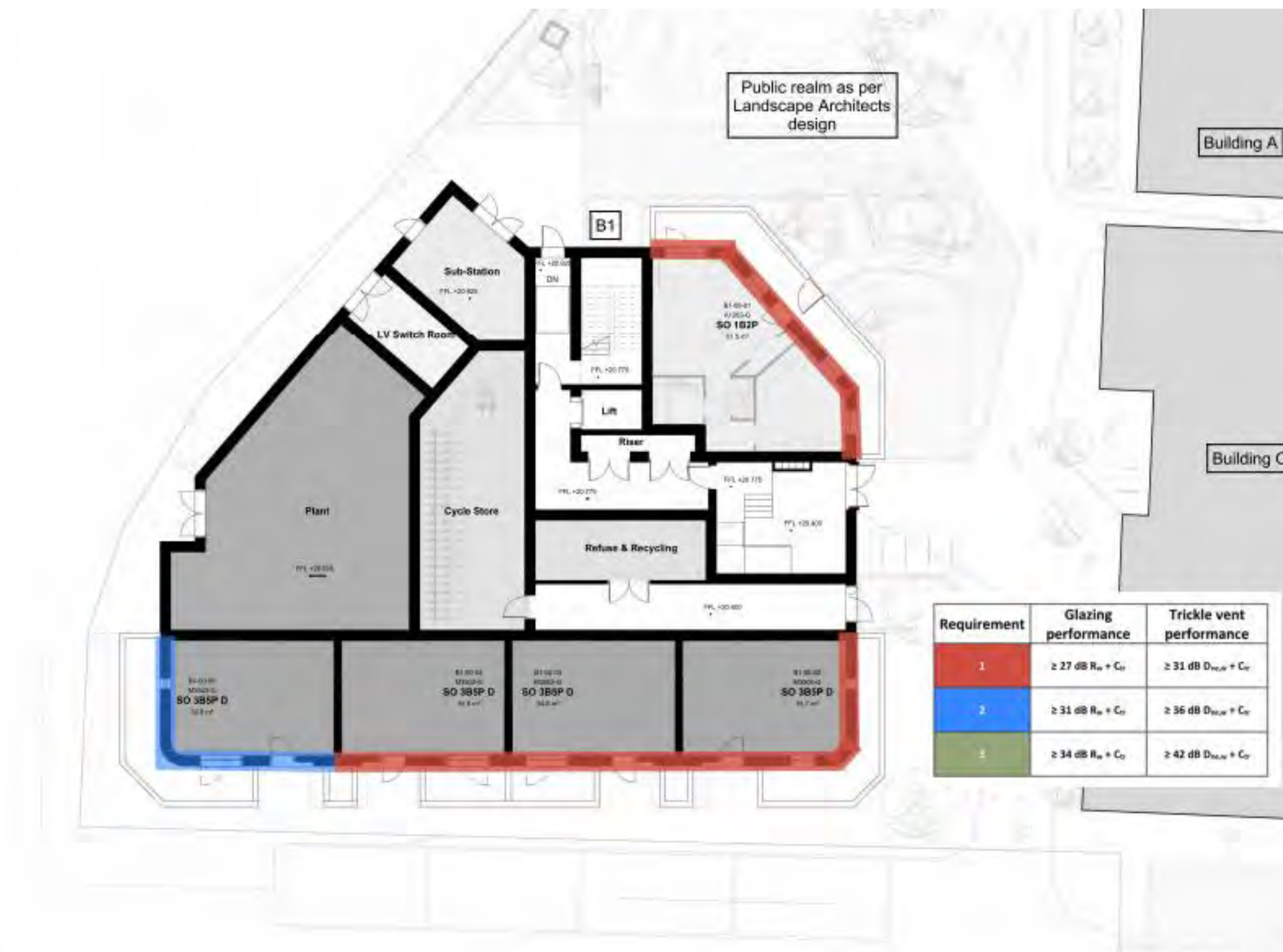
Figure 17: Façade acoustic performance requirements – Block B Level 0
