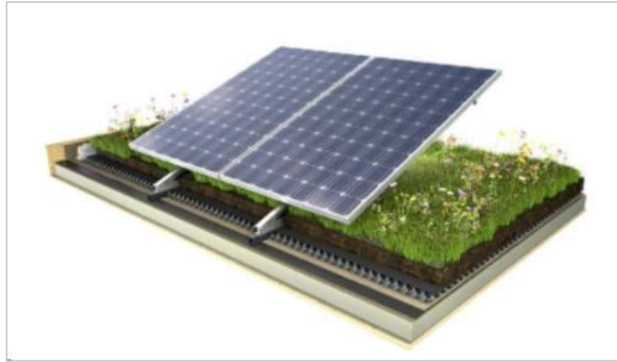
Figure 7-1: Bio solar roof.
