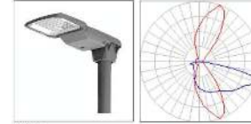
REF D: Kirium Pro S1, SLED, A1 Optic, 2.7K, 800mA. Complete with 35 Lux Photocell. Painted in Grey Ral 7046. 6M Tubular steel column. Galvanneal finish.
