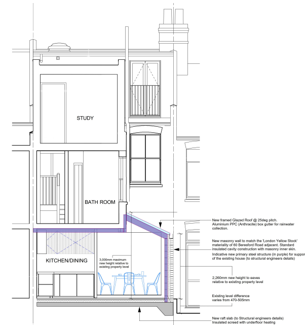
Figure 7. Section through proposed extension
