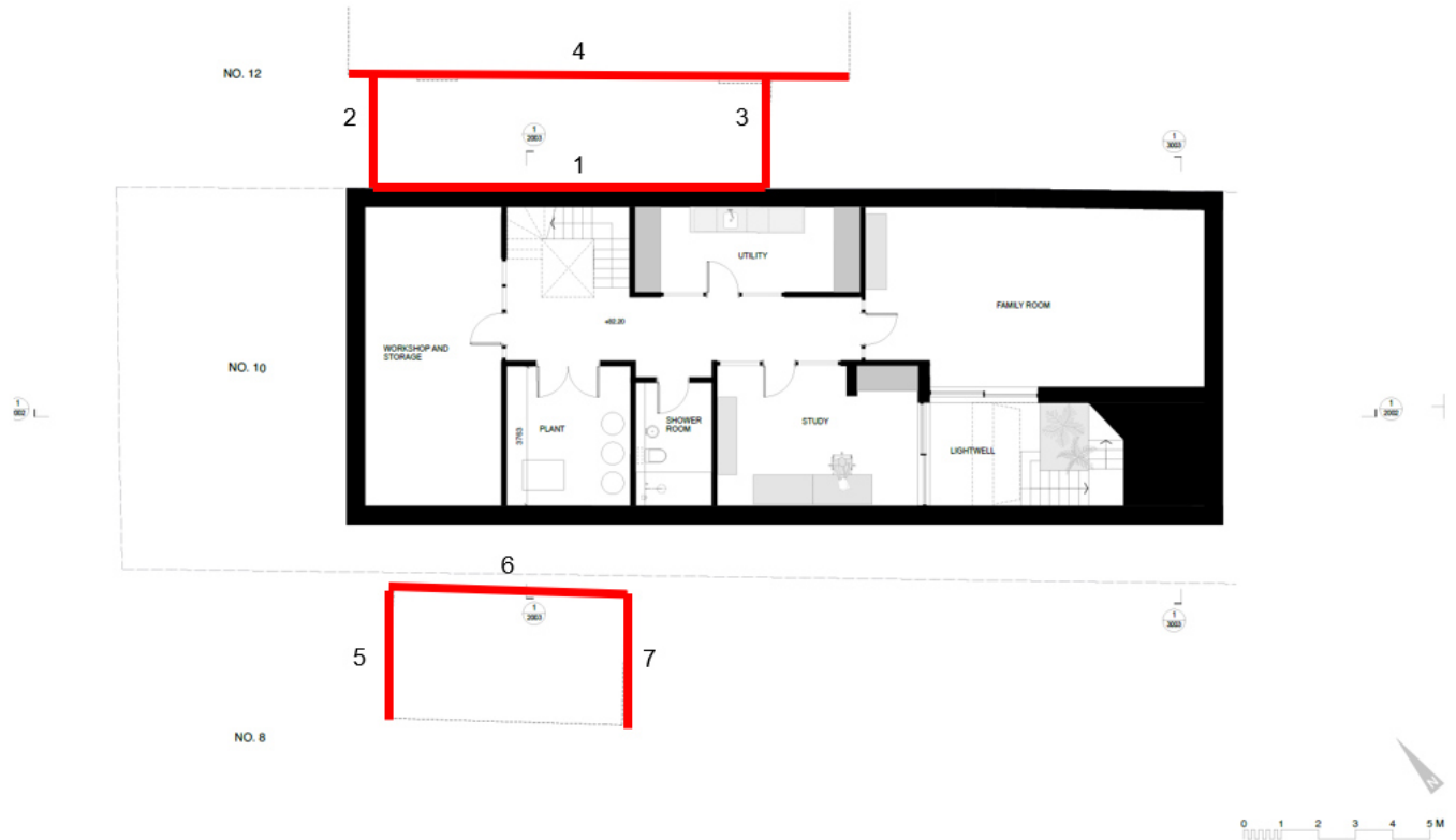
Figure 4.1 Plan view of 10 Fordington road with proposed basement overlay. Red highlighted walls have been analysed within 'Oasys XDISP' software. Drawing adapted from Yabsley Stevens Architects Drawing 10A1003
