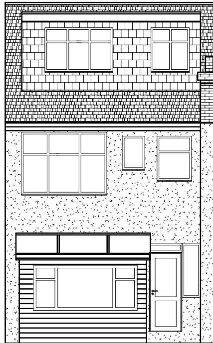
EXISTING REAR ELEVATION
