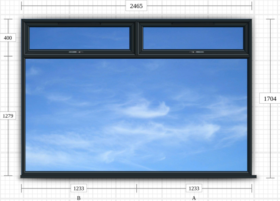
💡 Viewed from inside
