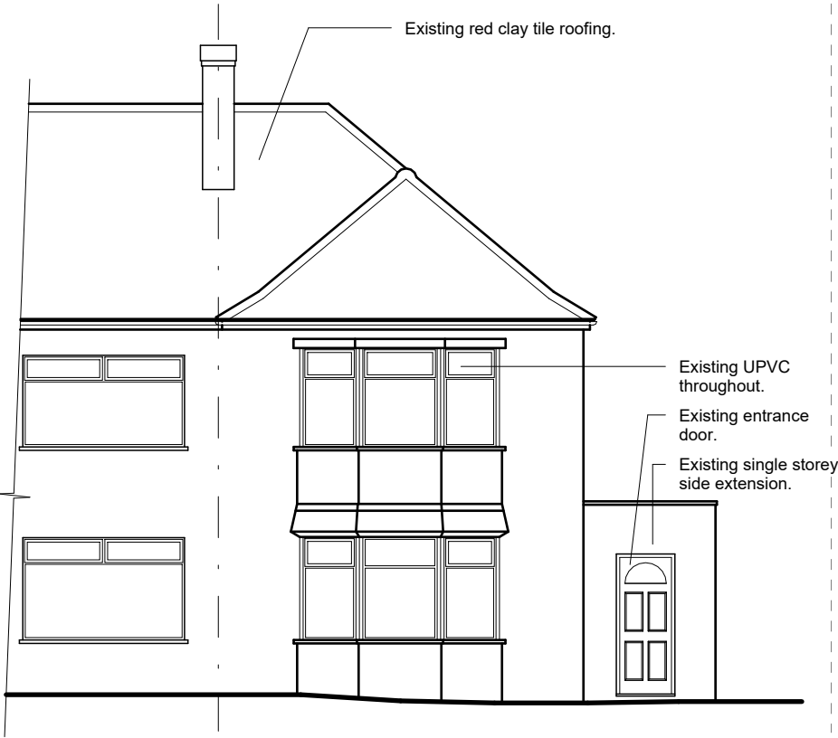
01 - Front elevation - existing
