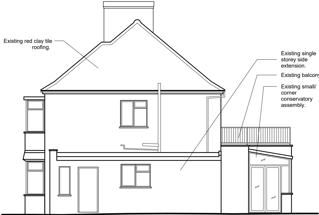
02 - Side elevation - existing
