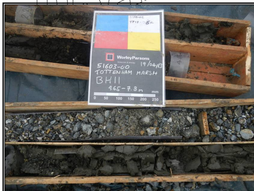
Plate 2. Kempton Park Gravels and London Clay recovered from BH11
