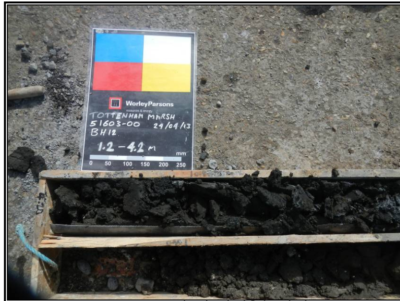
Plate 3. Made Ground and Alluvium recovered from BH12
