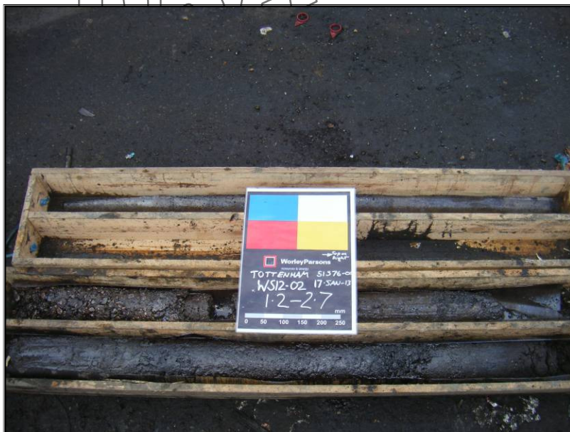
Plate 8. Soil arising from WS12-02 (1.2-2.7 mbgl) within the made ground, alluvium and Kempton Park Gravel. Hydrocarbon contaminants observed throughout core.
