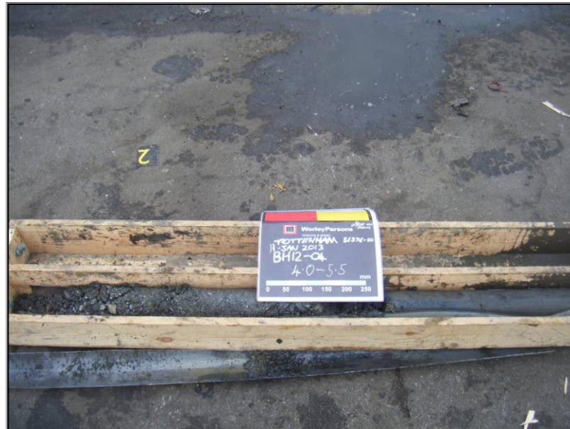
Plate 3. Soil arising from BH12-04 (4.0 to 5.5 mbgl) within Kempton Park Gravel.
