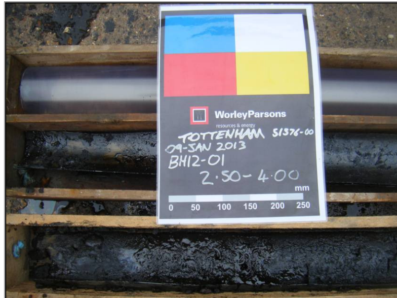
Plate 1. Soil arising from BH12-01 (2.5 to 4.0 mbgl) within made ground. Hydrocarbon staining apparent within sample.
