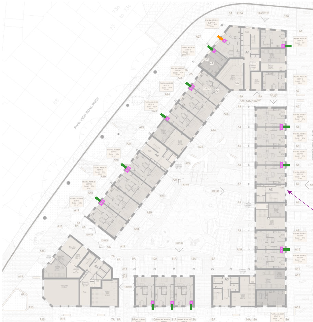
Ground floor for Building A showing location of the MVHR units and lengths of intake and exhaust ductwork to external wall. Lengths have been calculated based on the position of the MVHR unit and account for connections in and out of the MVHR unit.
