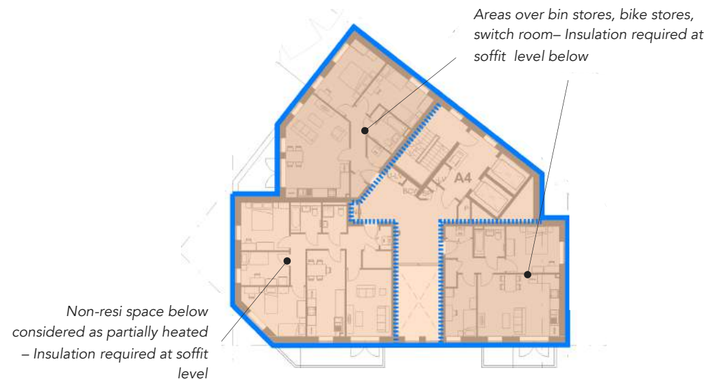
Block A4 - ground floor and first floor plan, depicting the thermal envelope
