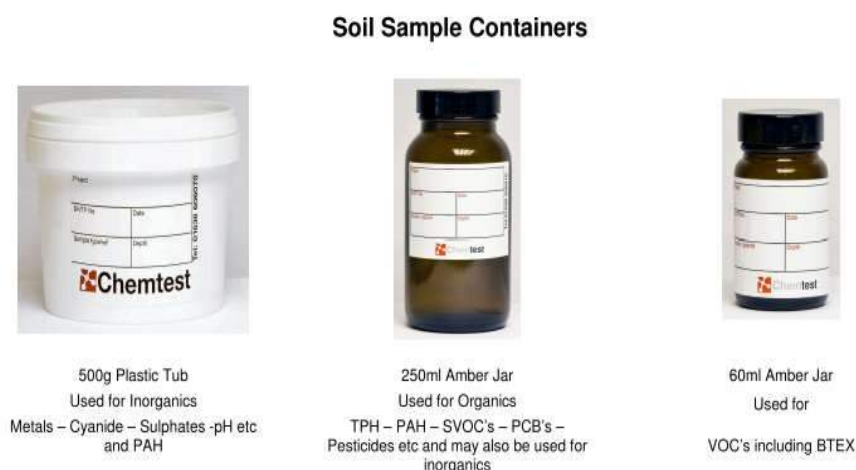
Figure 1 - Soil Sample Containers Required by Eurofin Chemtest
