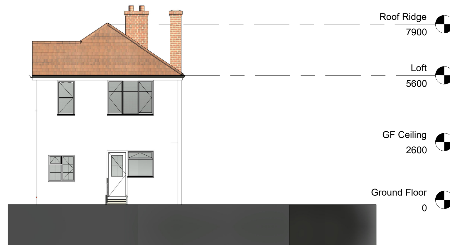
Existing East Elevation
