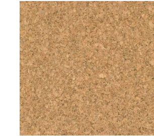
300X300 CORK FLOOR TILES IN ALL HABITABLE ROOMS ( ORIGINAL SPECIFICATION)
