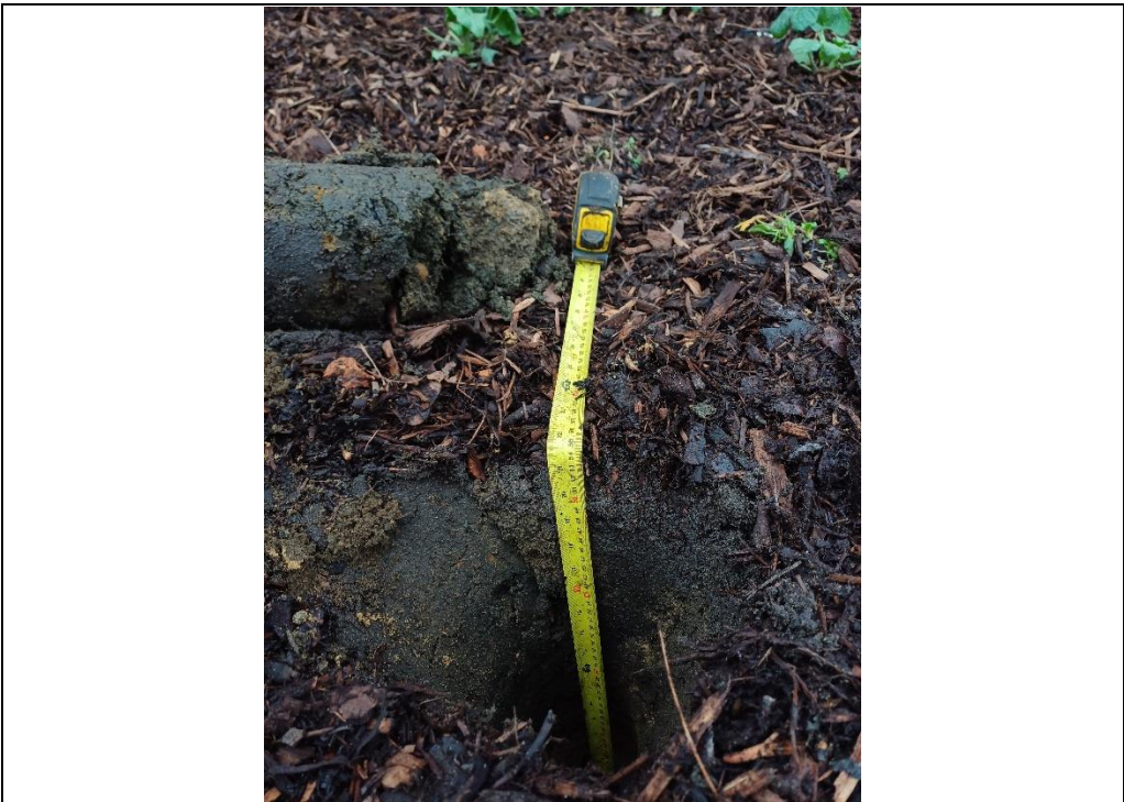
Plate 2: Street level planter – clean cover thickness.
