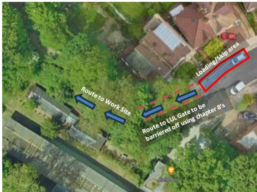
Site set up for deliveries and access routes on Priory Gardens road
