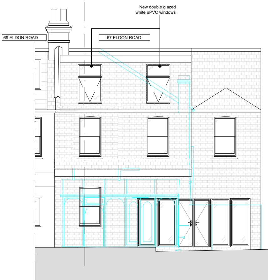
03 PROPOSED REAR ELEVATION 1:100@A3
