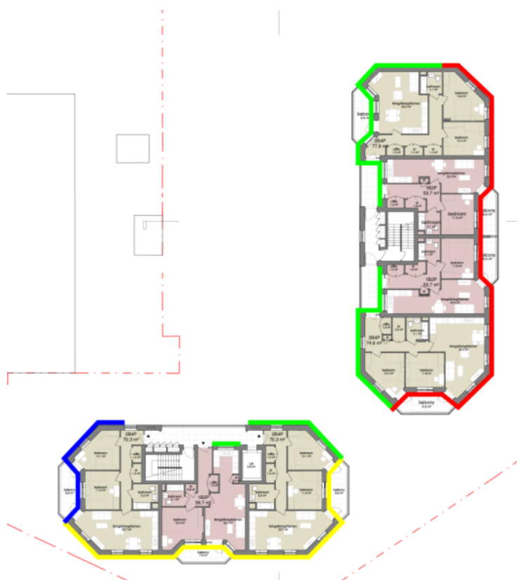
Figure 1: Façade identification of openable windows according to the acoustic report
