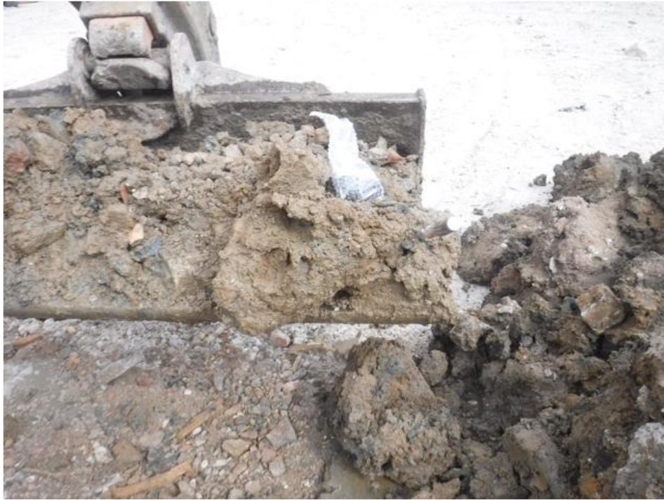
Validation Sample 'W. Sidewall' (2.90m). Soil directly below w. sidewall of Tank 4.
