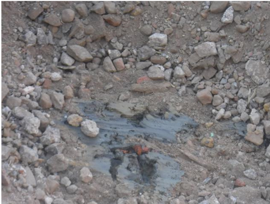
Cohesive Made Ground at 1.65m. Validation sample collected.
