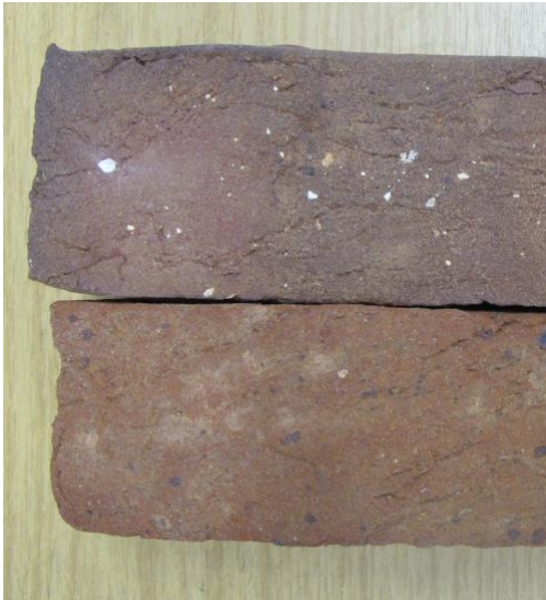
Image 14: Initial sample handmade bricks produced by Bulmer Brick and Tile to match existing
