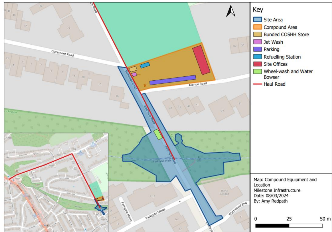
Figure 4: Haul route and site set up for Stanhope Road Bridge project
