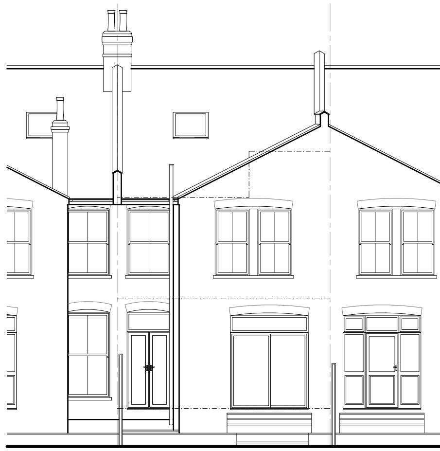
Rear Elevation As Existing 1:100
