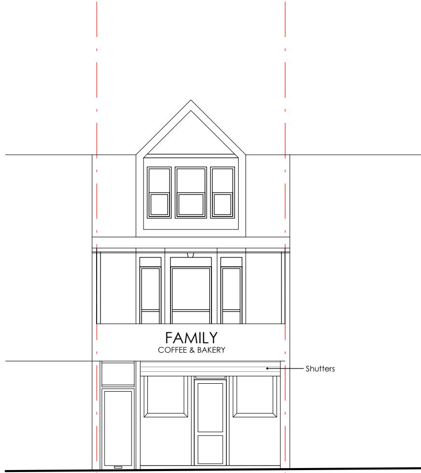
Shopfront Elevation As Proposed/As built
