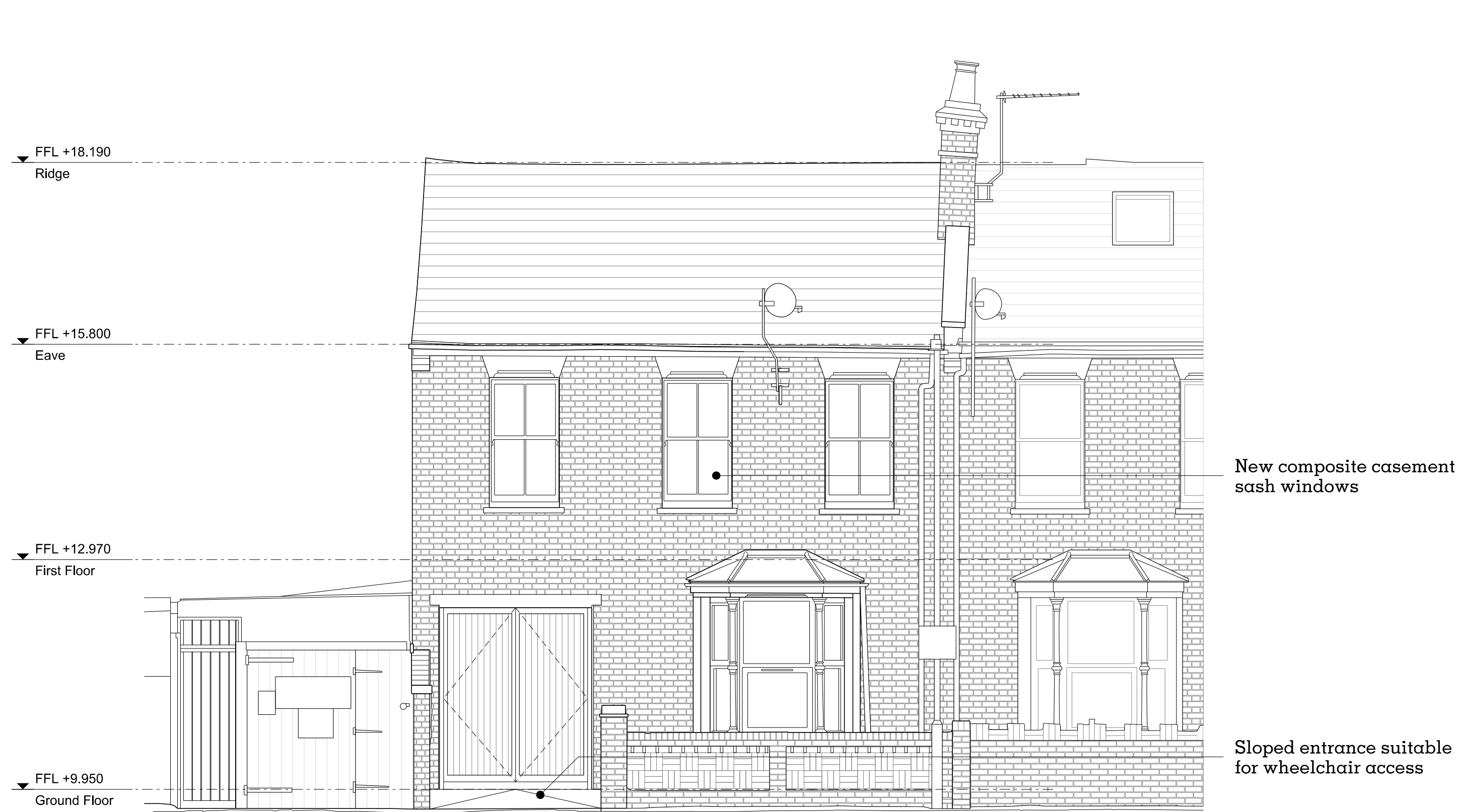
01 Proposed Front Elevation 1:50 @ A1
