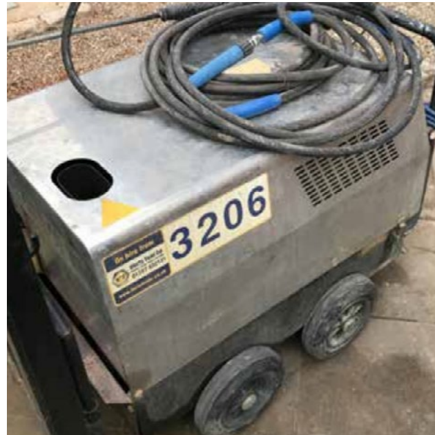
FIGURE 30. Proposed masonry cleaning machine to be used
