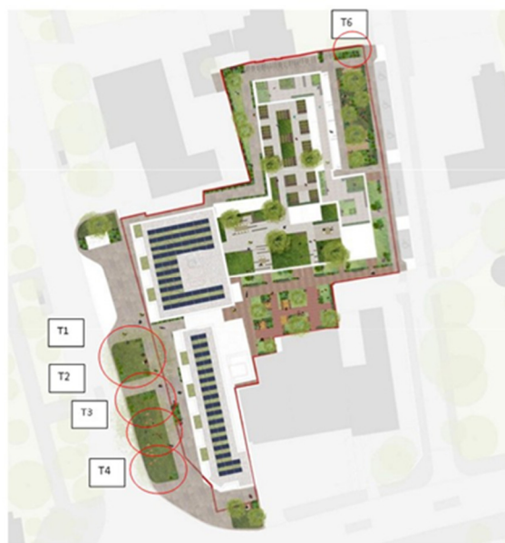
Above: Outline Concept design scheme showing the five retained tree locations in red.
