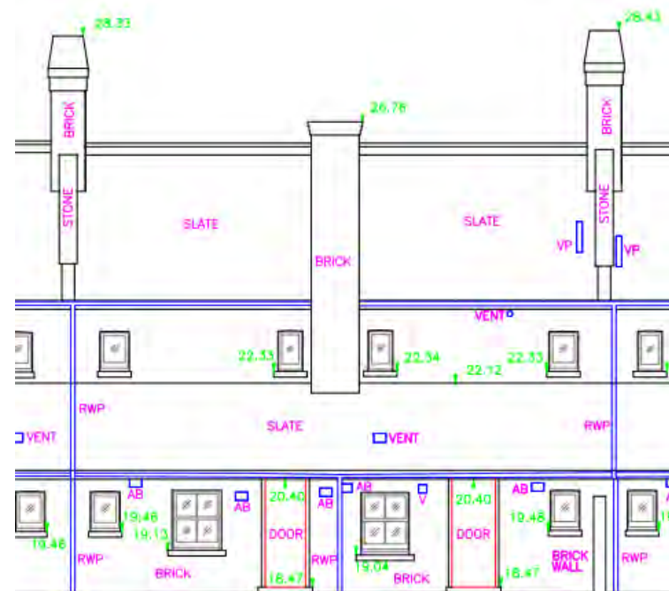
REAR ELEVATION EXISTING
