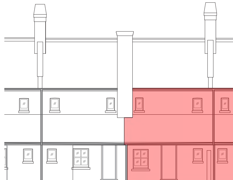
REAR ELEVATION DEMOLITION
