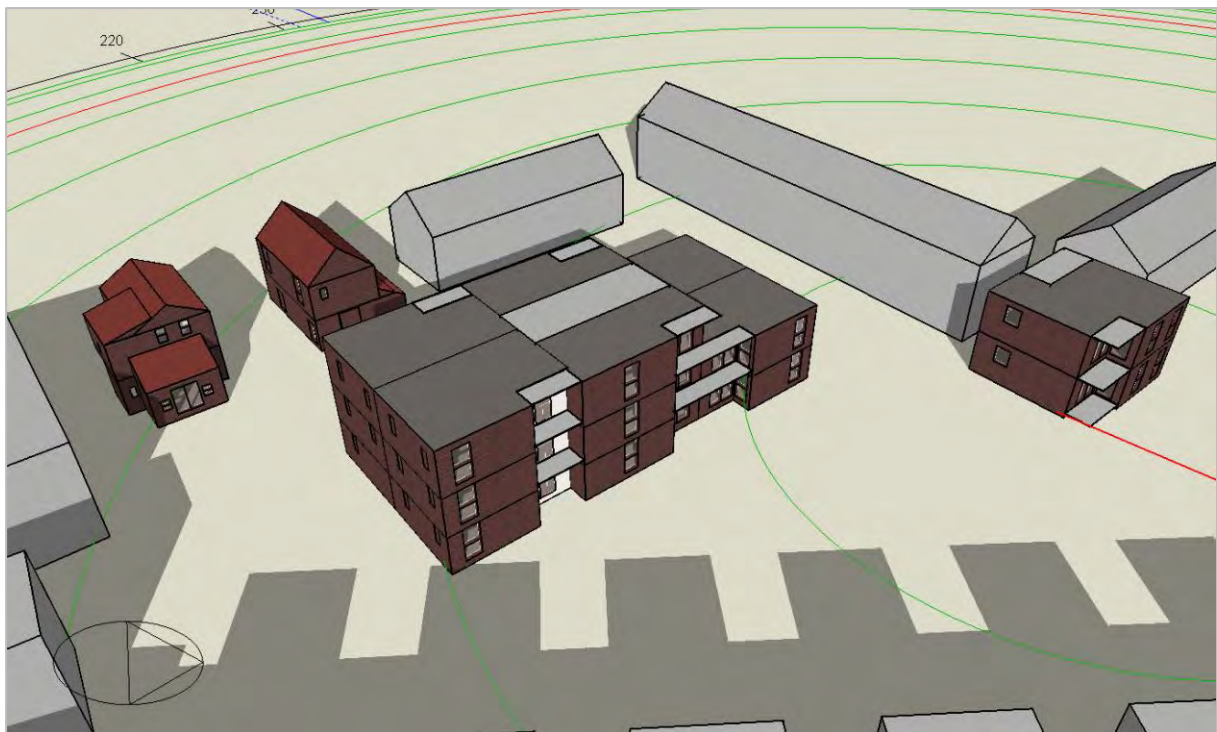
Figure 4: New dwellings simulation model from DesignBuilder for July 15 07:00.
