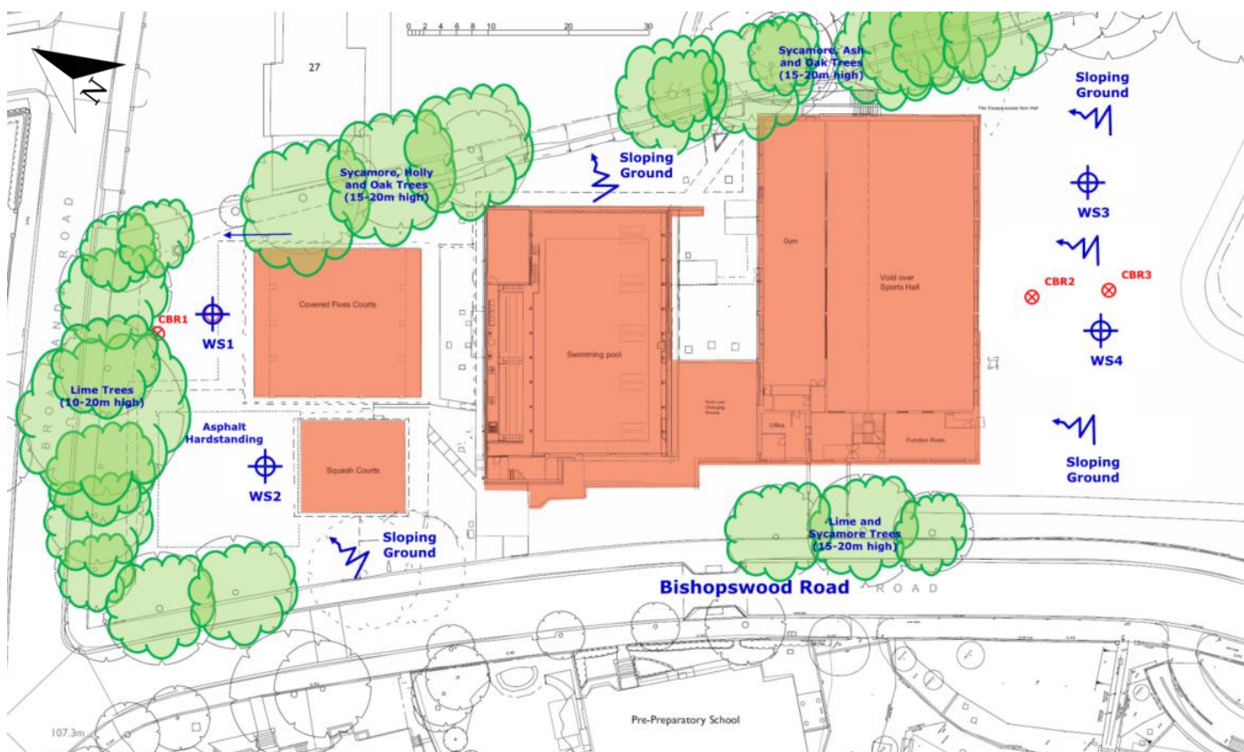
Figure 6.2 Ground investigation locations from the supplementary phase
